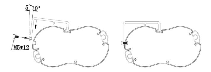
Fix on the base of front bar (according to the below drawing to drilling the holes which diameter is 14mm and the depth must be more than 80mm on the floor.)
