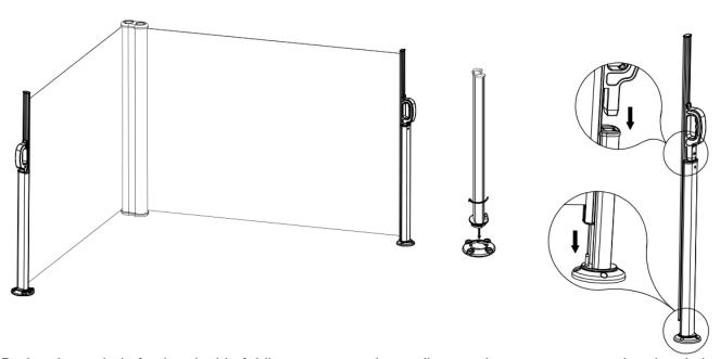
During the period of using double folding screen awning, pull out and retract, to ensure that the cloth surface and the ground parallel, otherwise the fabric will be twisted or not returned.
